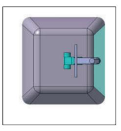
Top view of the cabin with the 2 racks removed for car storage in the garage
