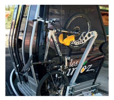
The CAB RACK is designed to safely transport 2 mountain bikes to the cabins. The mountain bikes are placed on the upstream and downstream sides of the cabins. The support structure consists of a cradle coming from underneath the cab. 2 racks (upstream and downstream) can be quickly removed to hold the mountain bike.
